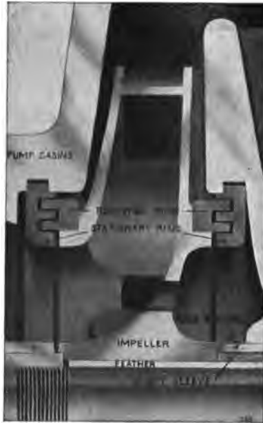
FIG. 202.—Detail of labyrinth rings in pump shown in Fig. 201.
